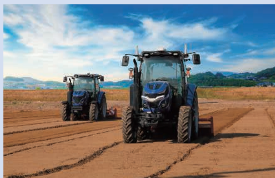
Collaborative operation using robot tractors
