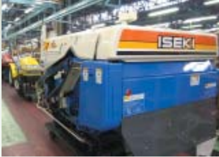
A mixed manufacturing system that enables combine harvesters and tractors to be assembled on the same production line (Iseki-Matsuyama Mfg. Co., Ltd.)
