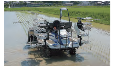
Manned monitoring-based robot rice transplanter
