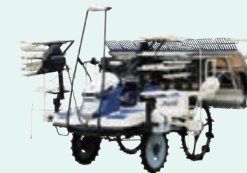
Rice transplanter equipped with straight travel/turning assist functions Sanae JapanPRJ18
