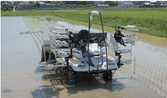
Manned monitoring-based robot rice transplanters which promote high expectations for further laborsaving
