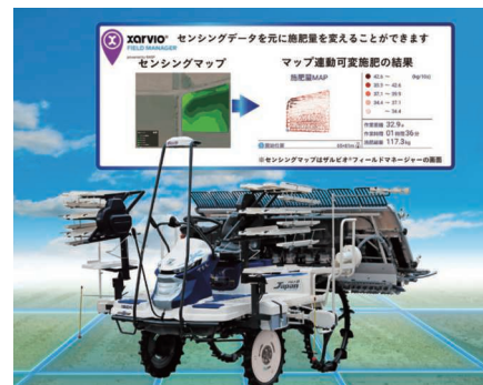
8-rows variable fertilizer rice transplanter PRJ-FV type
