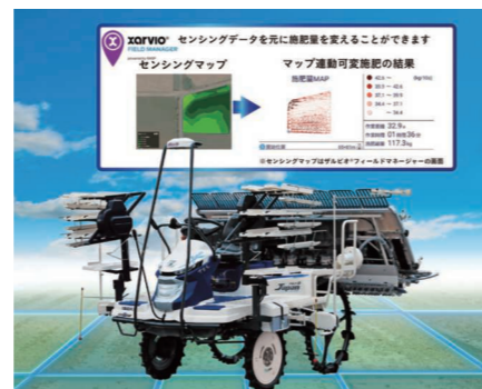
8-rows variable fertilizer rice transplanter PRJ-FV type
