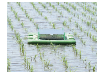
Aigamo-Robo, an automatic weeding robot
