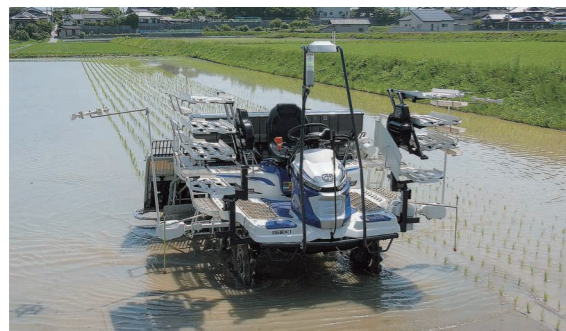
Manned monitoring-based robot transplanters which promote high expectations for further laborsaving
