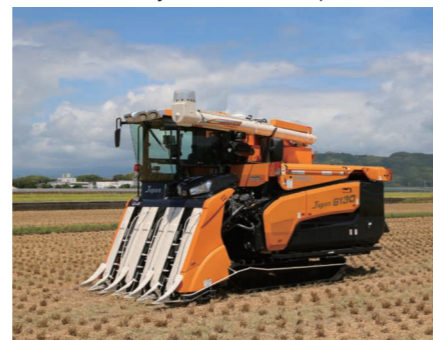
Six-row combine harvester HJ6130-Z, equipped with a function to assist straight traveling
