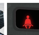
The system sets off a sound alarm with a light lit to warn that the seat belt is unfastened.
