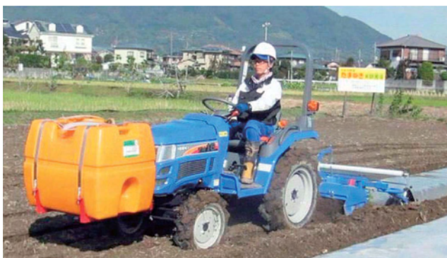
Herbicide application and ridge making at the same time
