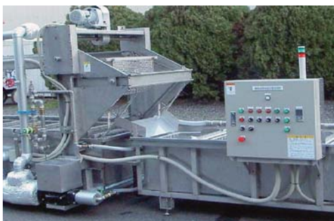
Hot-water disinfection facility
