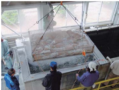
Hot-water disinfection facility with a seed bath
