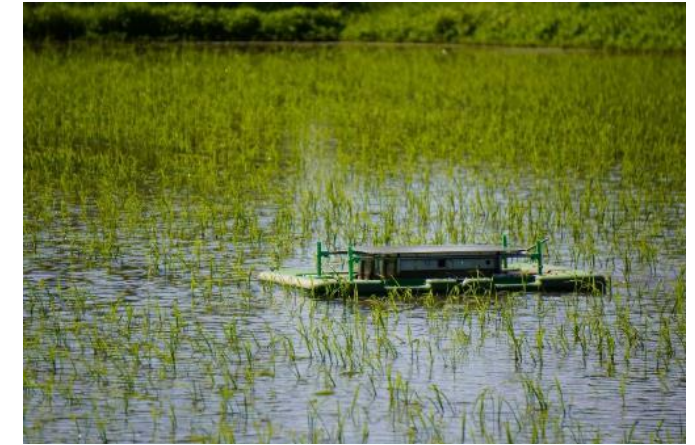
Aigamo-Robo operating in a paddy field
