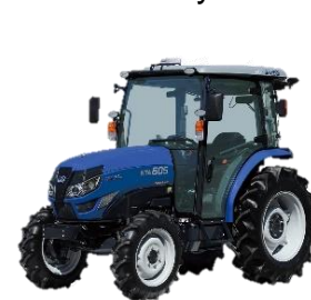
Mid-sized tractor with straight-travel assistance (36/50/60hp)
