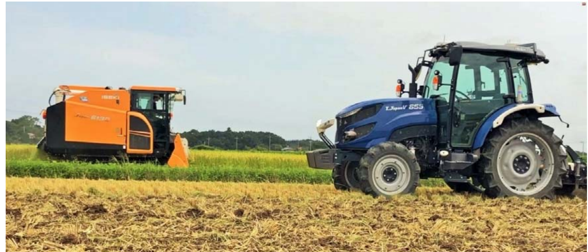
Improving work efficiency through the cooperative work of ISEKI's yield combine harvester and robot tractor
