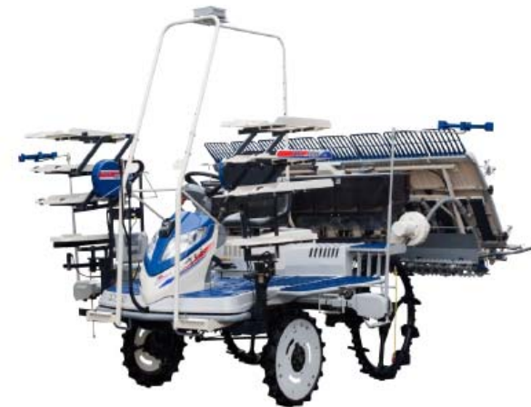
Rice transplanter with straight-travel assist system (To be released in Dec. 2017)
