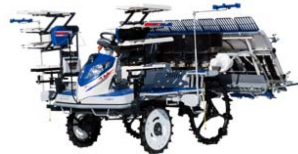
Variable fertilizing 8-row rice transplanter NP80-FV
