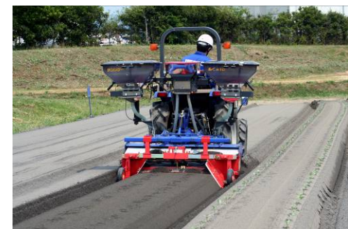
Inside ridge partial fertilizing machine (trapezoidal spec.)
