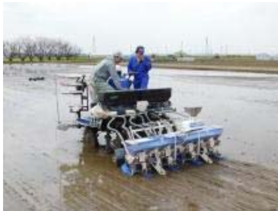
ICT rice transplanters (variable fertilizing and multi-purpose rice transplanters)
