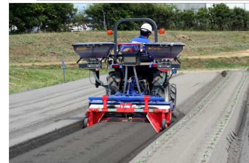
Inside ridge processor (trapezoidal spec)
