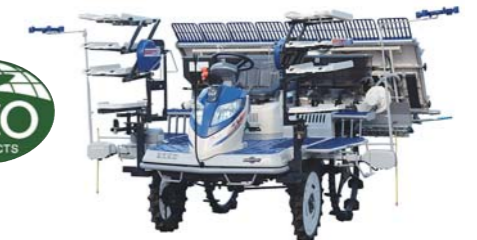
NP80D, variable fertilizing rice transplanter with soil sensor
