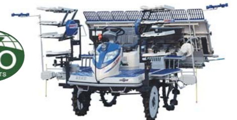
NP80D, variable fertilizing rice transplanter with soil sensor
